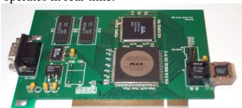
Figure 7: Photograph of the RTDS board.
