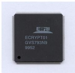
Figure 6: Photograph of the crypto processor.
