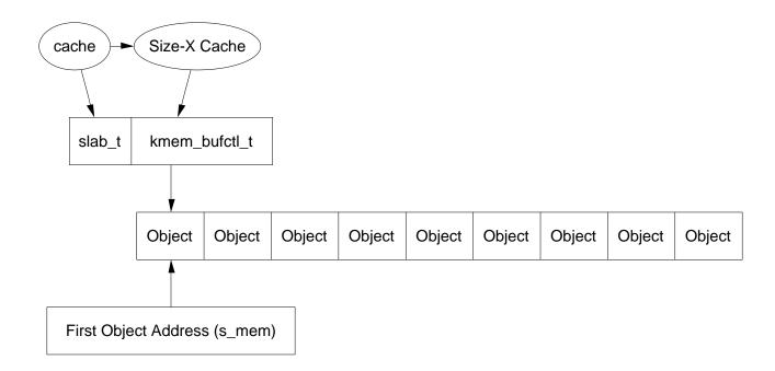
Figure 8.9: Slab With Descriptor Off-Slab
