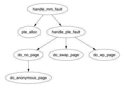
Figure 9.12: Call Graph: handle mm fault
