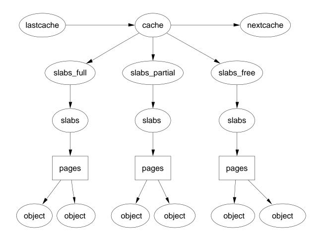
Figure 8.1: Layout of the Slab Allocator
