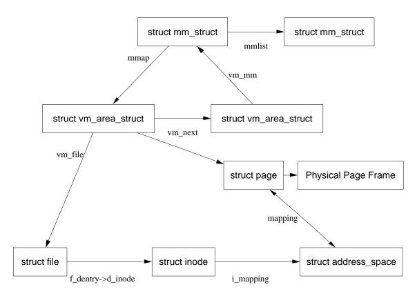
Figure 9.1: Data Structures related to the Address Space
