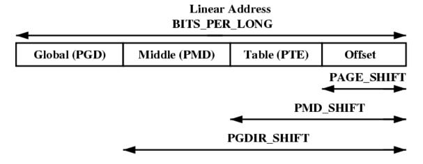
Figure 4.1: Linear Address Bit Size Macros
