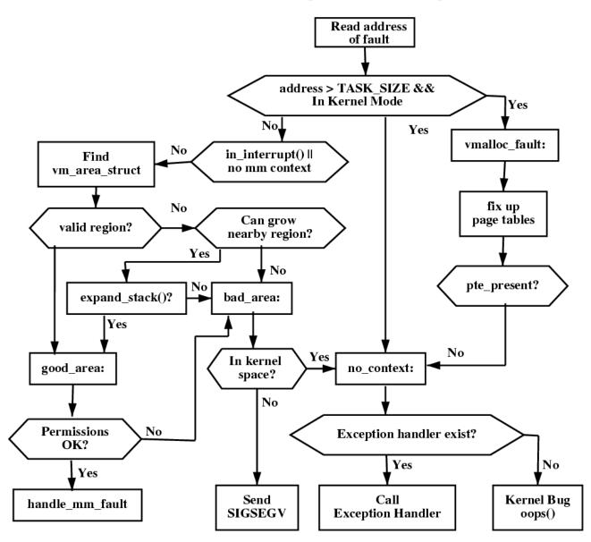
Figure 9.16: do\_page\_fault Flow Diagram
