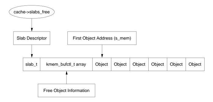
Figure 8.8: Slab With Descriptor On-Slab
